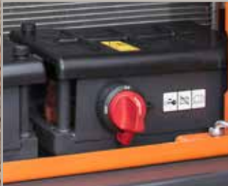
Battery cut-off switch
