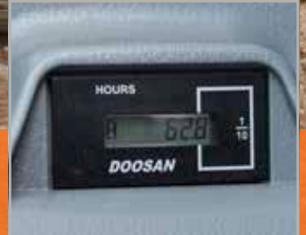
Hour meter (from ground level)
