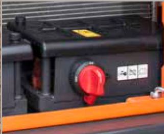
Battery cut-off switch
