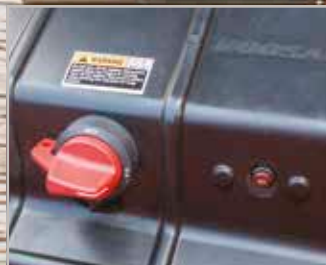
Battery cut-off switch
