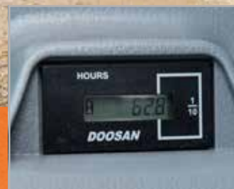
Hour meter (from ground level)
