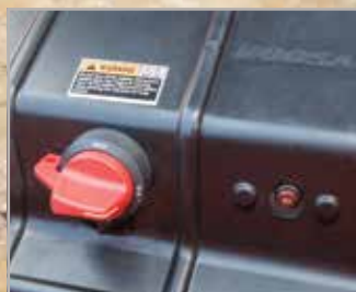
Battery cut-off switch
