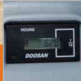
Hour meter (from ground level)
